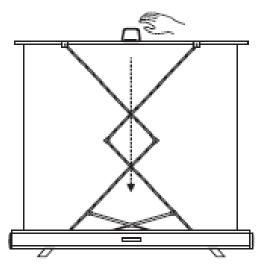
Tip: If the screen does not go in the cradle, lift it up and maneuver it inside.
