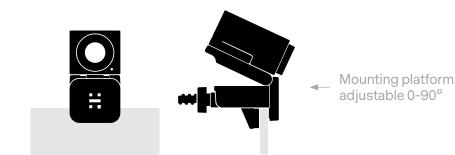
Bracket with camera mounted on display
